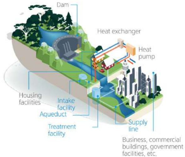
Concept Diagram of Hydrothermal Energy
